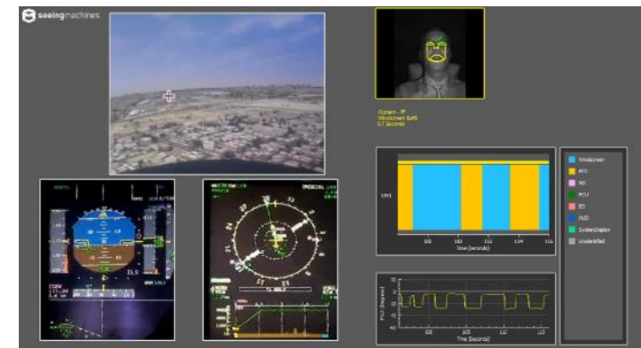
Example CandyBar™ multi-crew attention-time plot against customisable Areas of Interest, event markers, and time periods.
